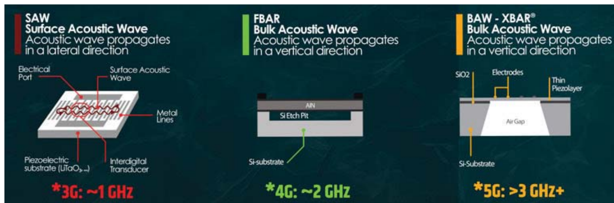
2. The XBAR resonator's structure (right) results in a bulk-acoustic-wave device that requires few manufacturing steps to fabricate RF filters.
